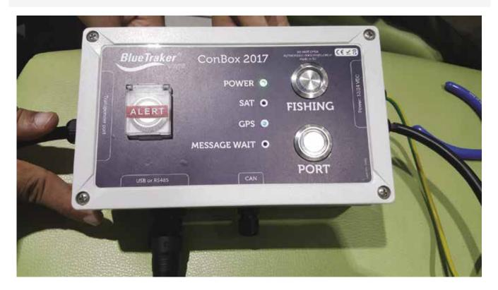
An example of a new Gen 2 unit incorporating new port, fishing, and SOS alert functions.
