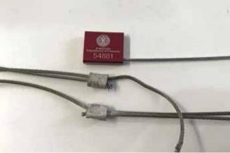
These photos show the steel locking mechanism attached to a VMS MTU (left) and a degraded lock (right).
