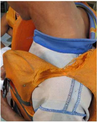
These two photos show the degradation over time of lifejackets stored on-board fishing vessels. It is important that these are checked regularly to ensure that they are still fit for purpose.
